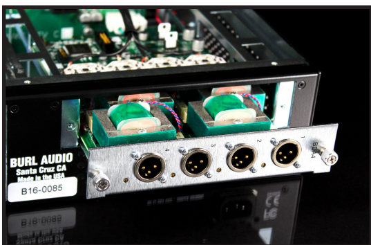
Image 7: With the B16 cover removed, install the BAD4M into the card guides as shown (BDA4M shown here). Make sure the metal Daughter Card backplate, not PCB, is inserted into the card guides.
